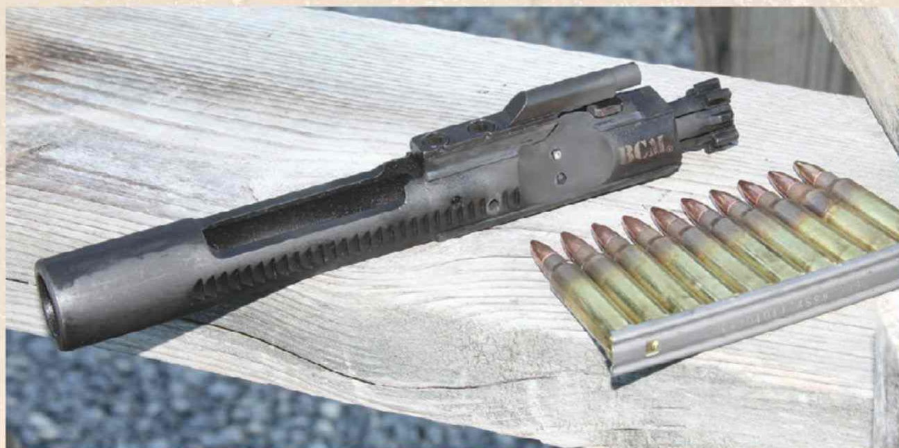
At 1,000 rounds of XM193, bolt retained very little carbon and most of the FireClean.
