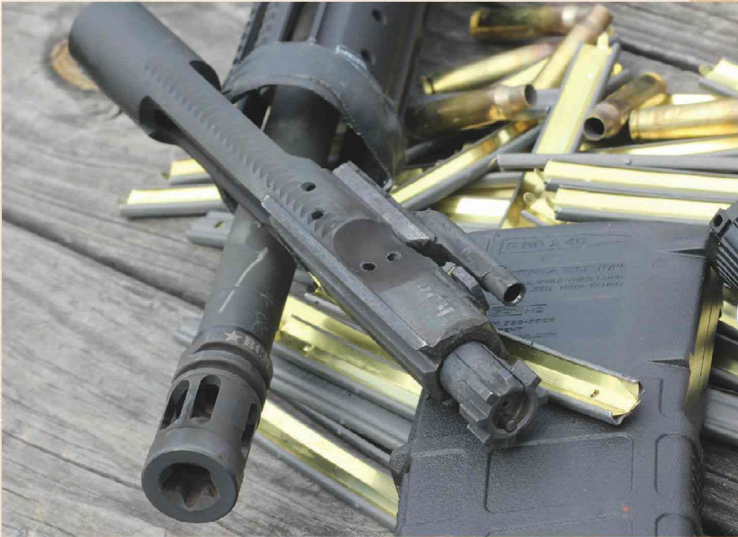
At 3,000 rounds, bolt group was dirty but cycled without complaint.
