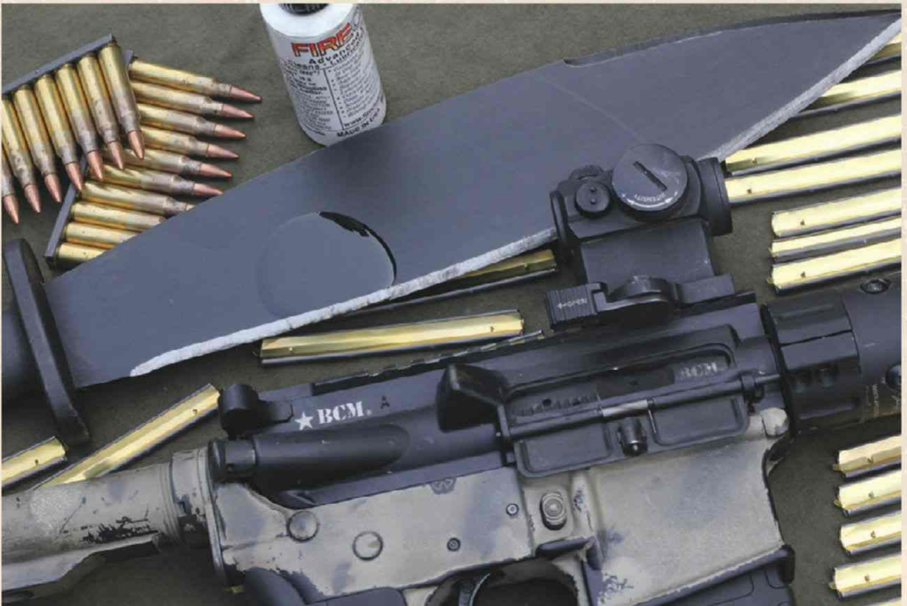
FireClean recommends 20 to 28 drops—amount shown on this blade—to treat an entire AR. A little goes a long way and lasts.
