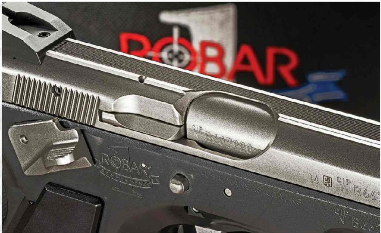
Above: ROBAR relieved ejection port for more positive ejection.
