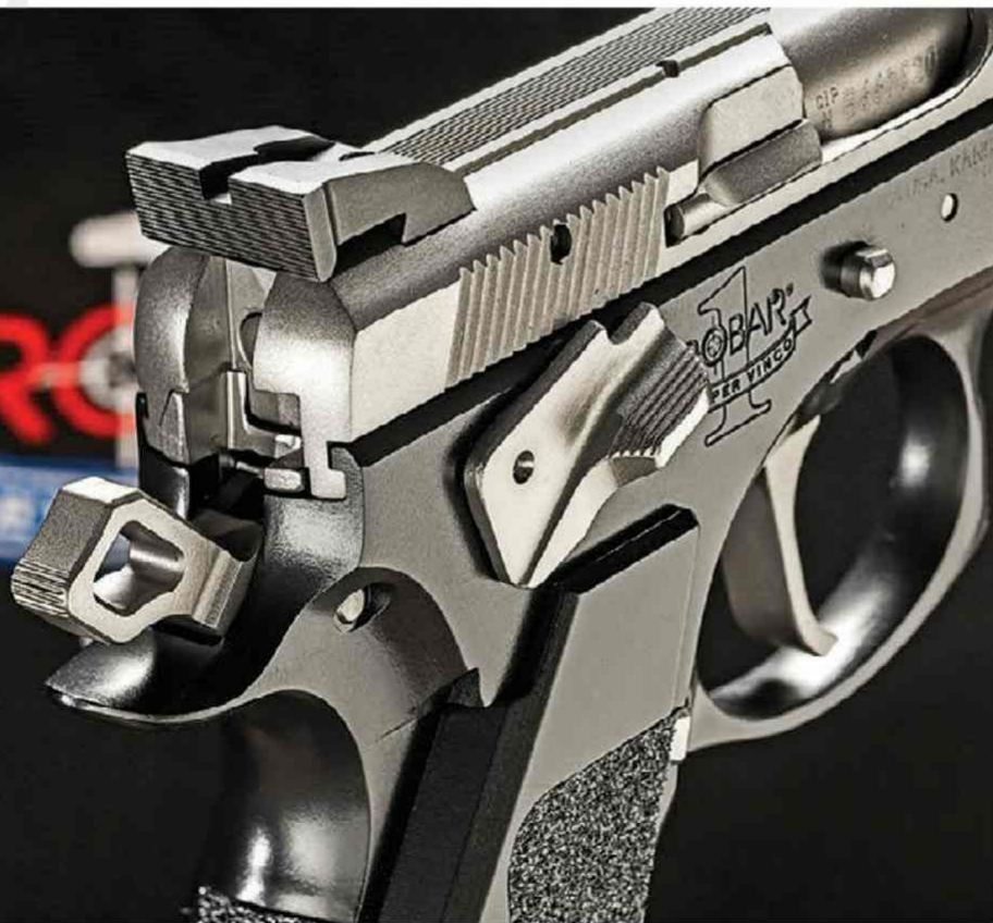
Below: ROBAR installed CZ Custom Shop competition sights and ambidextrous thumb safety.
